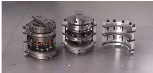
Quick Change Tool Cassettes hold the punch, die and stripper. They are set off-line so as to not limit machine run time.
