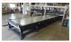
At 10.5M (34.4') long, will hold 3 full 5x10 sheets of material up to 1.0" and facilitates lean manufacturing by allowing de-nesting in the same order as cutting. Also available in standard duty, non-marring belt type.
