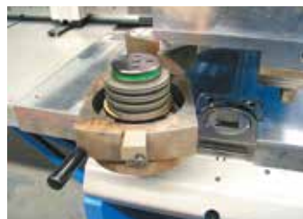
Boschert 4-way and 7-way RevoTool punch heads and die bases. Complete tool sets of customer choice are included.
